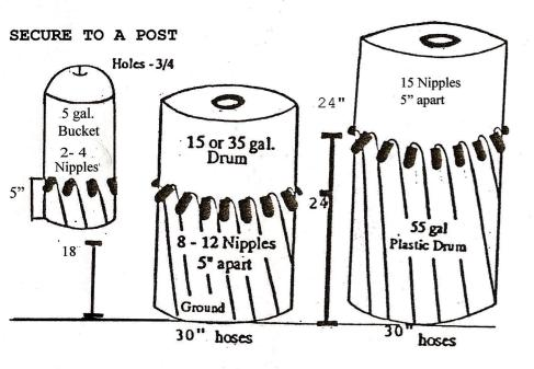
35 or 55 gal Drums on Wheels-15 Nipples each with 24" PVC hoses
